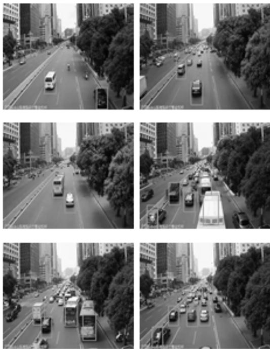
图 7 特定运动区域的 SEMI-SVM 车辆检测结果 Fig.7 Vehicle detect results of specific motion region based on SIMI-SVM
