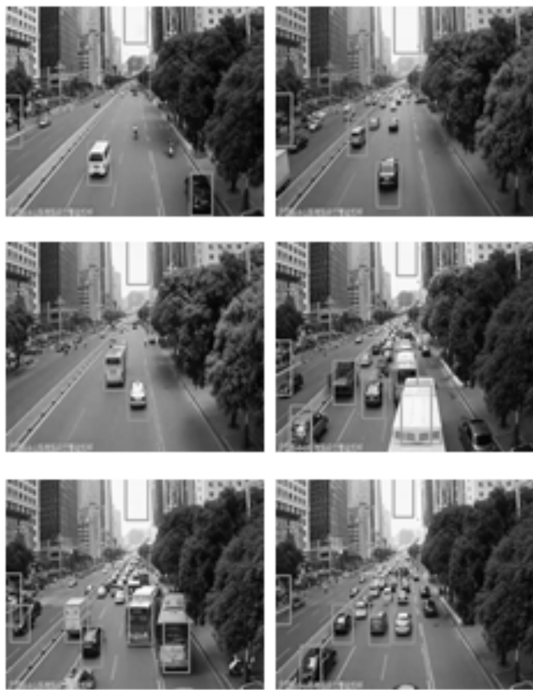
图 6 半监督学习后分类器的车辆检测结果 Fig. 6 Vehicle detect results after semi-supervised learning
