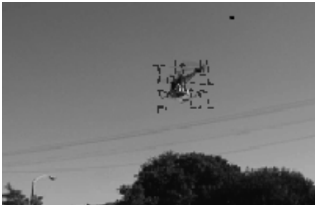
图 4 初始帧目标区域随机采样 Fig.4 Random sampling around the target in the first frame
