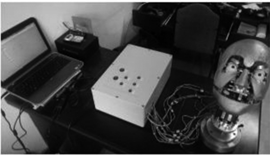
图 6 具有面部表情的仿人头部机器人系统 Fig.6 The system of humanoid robot head with facial expression
