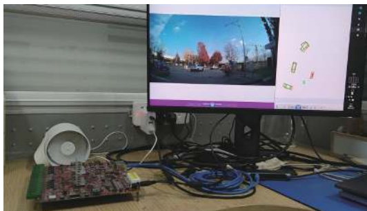
图9 面向车规级芯片的对象检测模型验证系统 Fig. 9 Object detection model verification system for car-level chips
