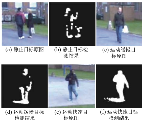
图 2 混合高斯模型对不同运动状态目标的检测结果 Fig. 2 Detection results of Gaussian mixture model for objects in different moving states
