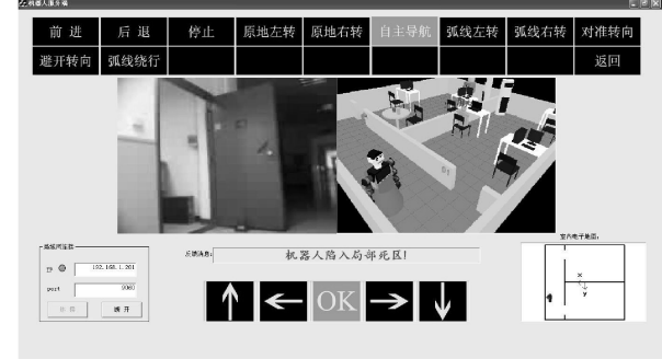
图 10 机器人陷入局部死区时的人机界面 Fig.10 The HRI whils the robot is trapped into a blind area
