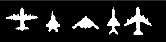
图 7 从卫星图片中分割出的 5 种型号飞机形状 Fig.7 The 5 kinds of plane contour divided from sensing images
